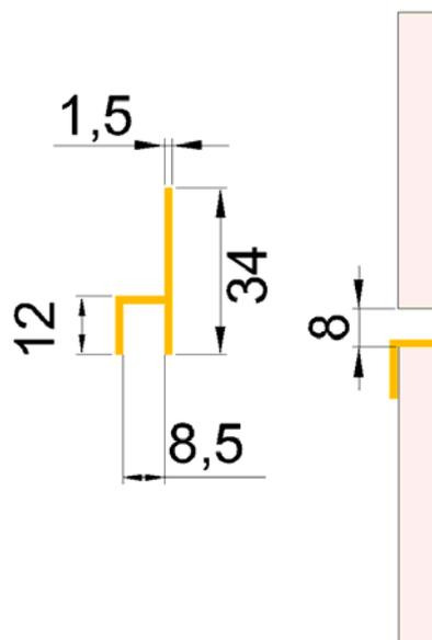
Figure 5 - Exemple de joint horizontal
