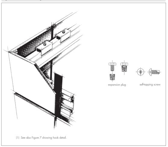
1.9 Two types of screw are approved for fixing the panels to timber battens, ie powder-coated for quick assembly and self-centreing with a separate washer and cap. The cover caps and powder-coated screws are available in colours to match the panel (see Figure 1 and Table 2).
